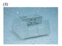
The aluminum load cell of the SJ-WP series is treated with alumite and silicon to be anti-corrosive and withstand long-term use in wet environments.
