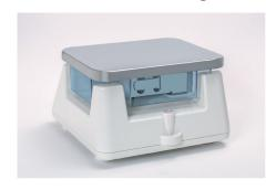
This innovative design allows the device to be completely sealed from moisture without compromising the weighing speed and stability due to up and down movement of the load cell changing the air pressure inside. As a result, the SJ-WP series can **stabilize in 0.5 seconds or less\***<sup>3</sup>, which further helps to improve factory productivity and efficiency.
